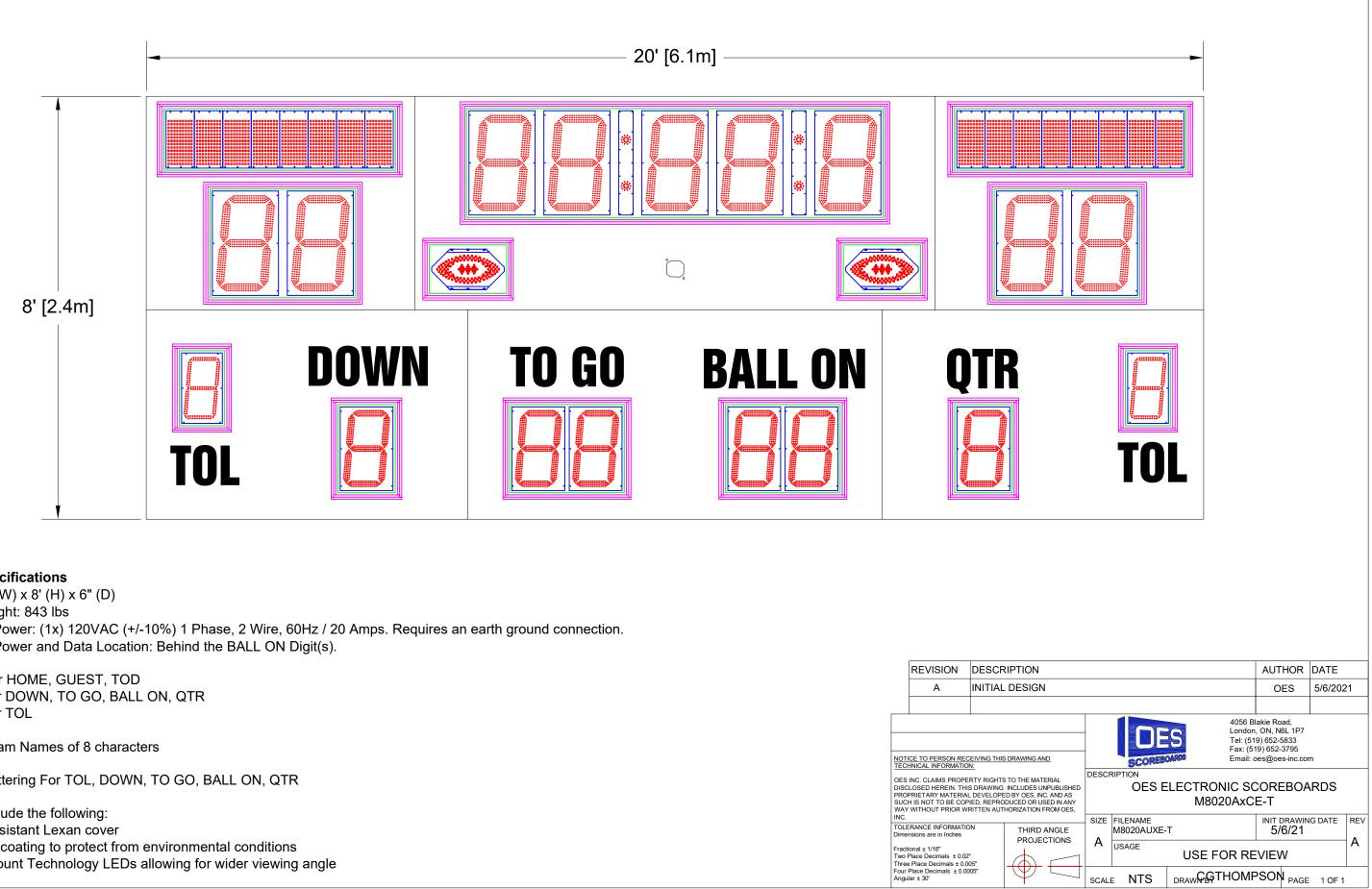
Overall size: 20' (W) x 8' (H) x 6" (D) Approximate Weight: 843 lbs Incoming Mains Power: (1x) 120VAC (+/-10%) 1 Phase, 2 Wire, 60Hz / 20 Amps. Requires an earth ground connection. Incoming Mains Power and Data Location: Behind the BALL ON Digit(s).
