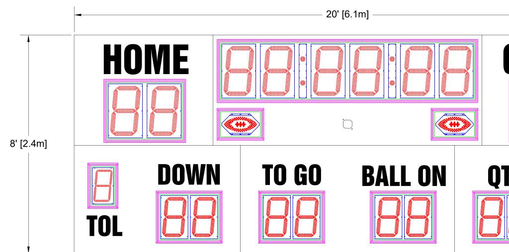
Overall size: 20' (W) x 8' (H) x 6" (D) Approximate Weight: 822 lbs Incoming Mains Power: (1x) 120VAC (+/-10%) 1 Phase, 2 Wire, 60Hz / 20 Amps. Requires an earth ground connection. Incoming Mains Power and Data Location: Behind the BALL ON Digit(s).
