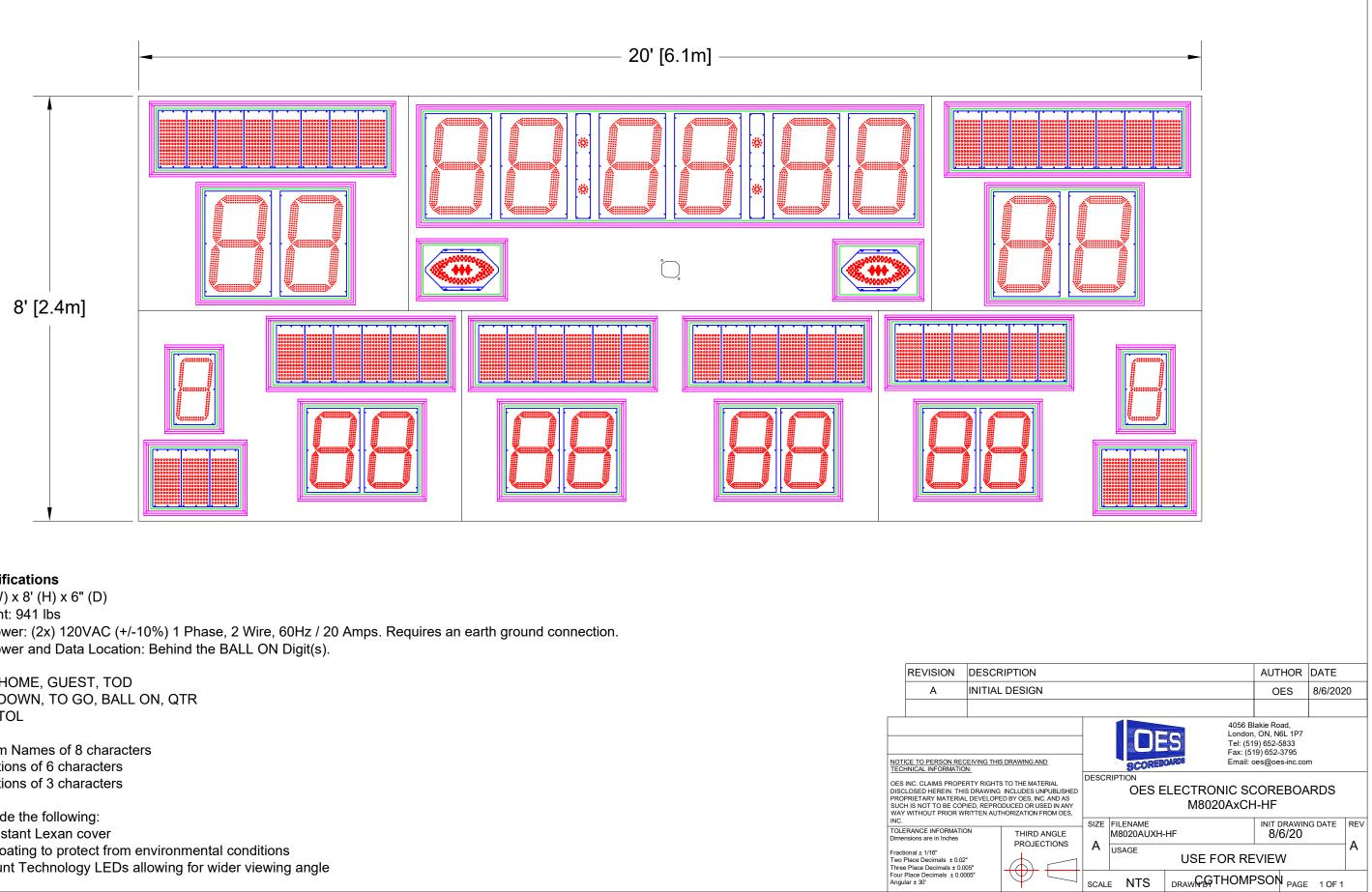
Overall size: 20' (W) x 8' (H) x 6" (D) Approximate Weight: 941 lbs Incoming Mains Power: (2x) 120VAC (+/-10%) 1 Phase, 2 Wire, 60Hz / 20 Amps. Requires an earth ground connection. Incoming Mains Power and Data Location: Behind the BALL ON Digit(s).
