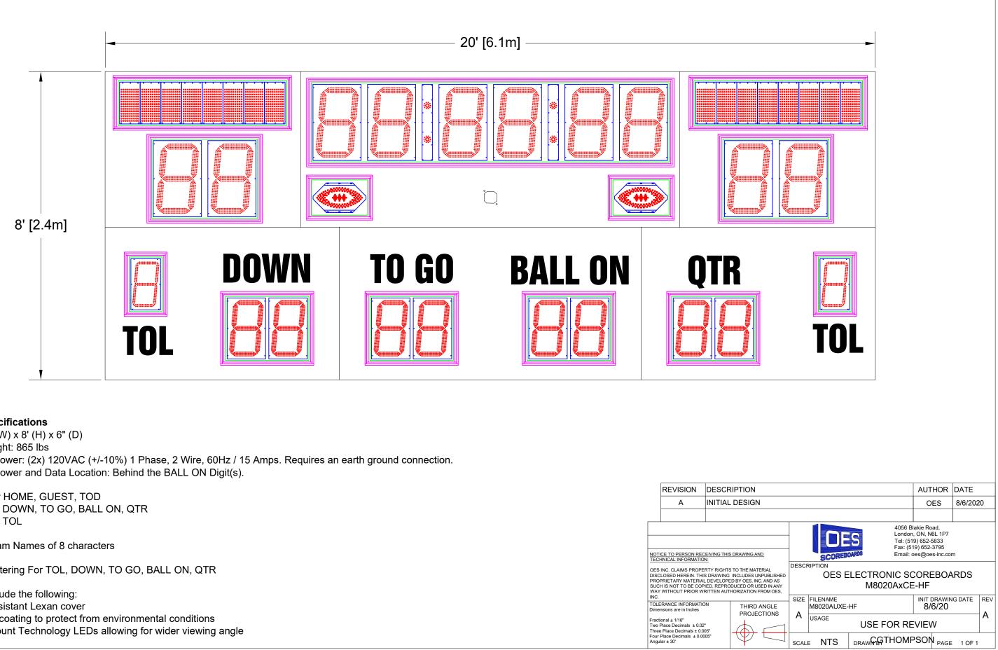
Overall size: 20' (W) x 8' (H) x 6" (D) Approximate Weight: 865 lbs Incoming Mains Power: (2x) 120VAC (+/-10%) 1 Phase, 2 Wire, 60Hz / 15 Amps. Requires an earth ground connection. Incoming Mains Power and Data Location: Behind the BALL ON Digit(s).
