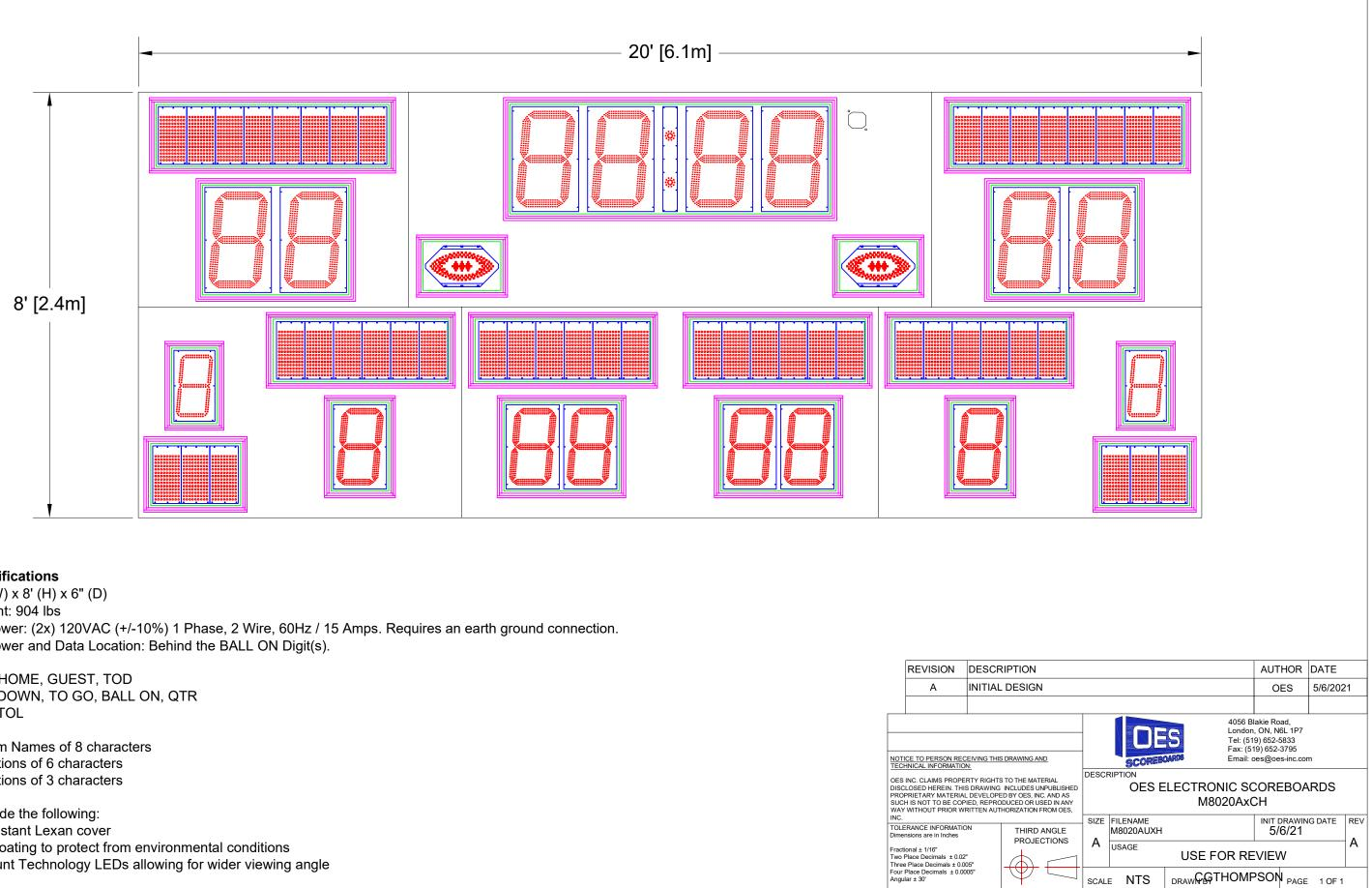
Overall size: 20' (W) x 8' (H) x 6" (D) Approximate Weight: 904 lbs Incoming Mains Power: (2x) 120VAC (+/-10%) 1 Phase, 2 Wire, 60Hz / 15 Amps. Requires an earth ground connection. Incoming Mains Power and Data Location: Behind the BALL ON Digit(s).
