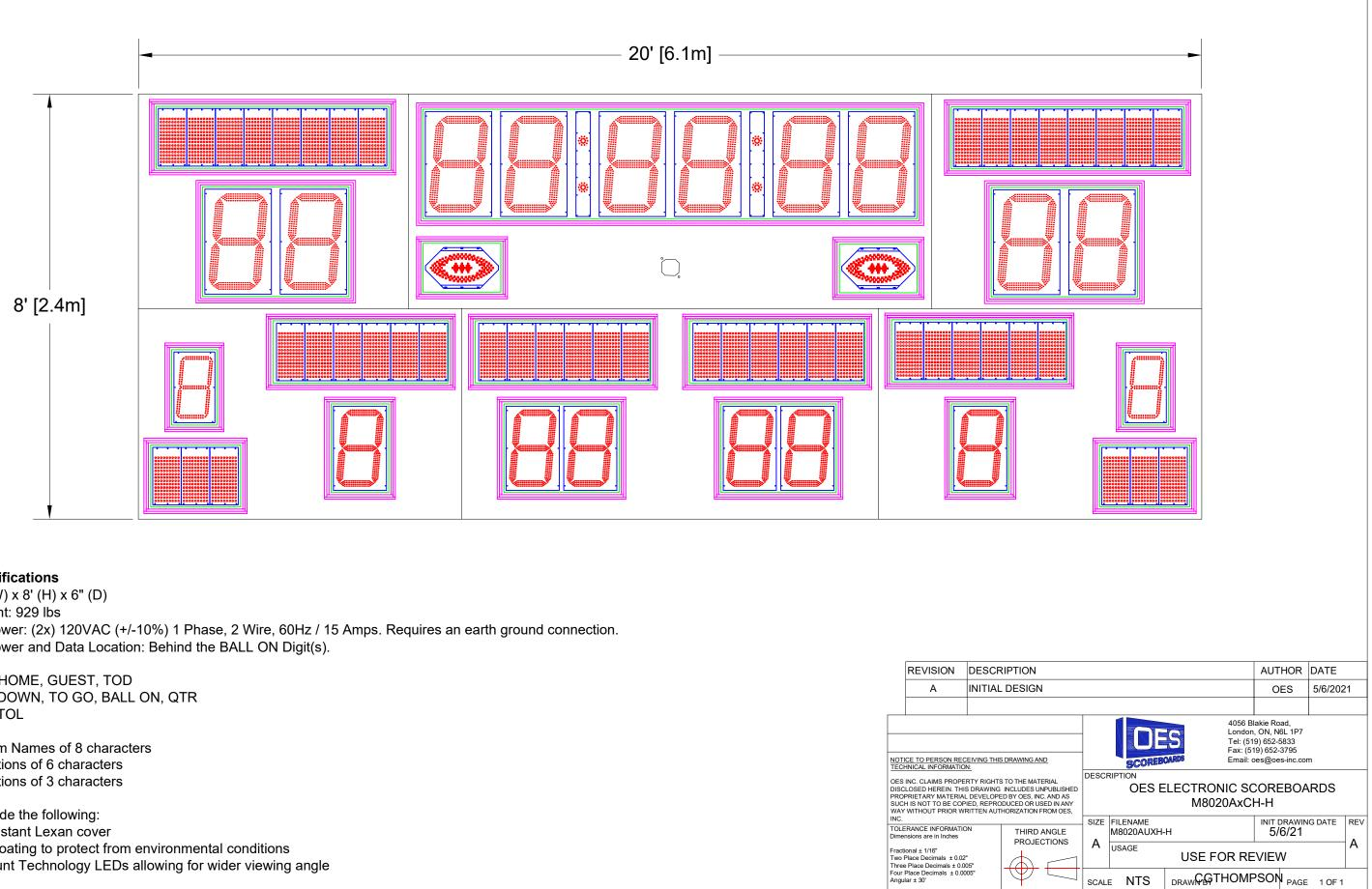
Overall size: 20' (W) x 8' (H) x 6" (D) Approximate Weight: 929 lbs Incoming Mains Power: (2x) 120VAC (+/-10%) 1 Phase, 2 Wire, 60Hz / 15 Amps. Requires an earth ground connection. Incoming Mains Power and Data Location: Behind the BALL ON Digit(s).
