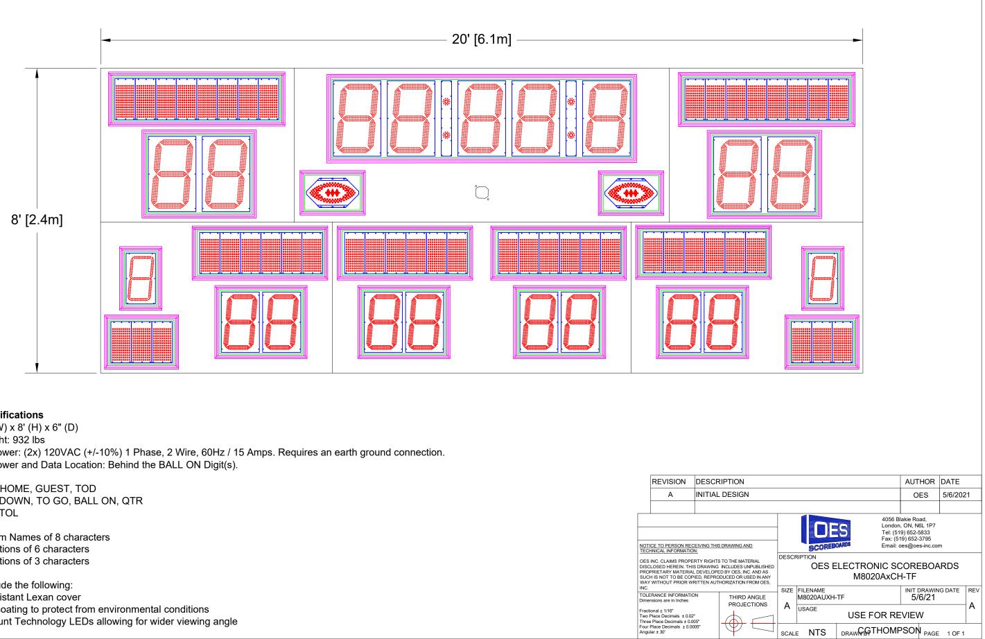
Overall size: 20' (W) x 8' (H) x 6" (D) Approximate Weight: 932 lbs Incoming Mains Power: (2x) 120VAC (+/-10%) 1 Phase, 2 Wire, 60Hz / 15 Amps. Requires an earth ground connection. Incoming Mains Power and Data Location: Behind the BALL ON Digit(s).
