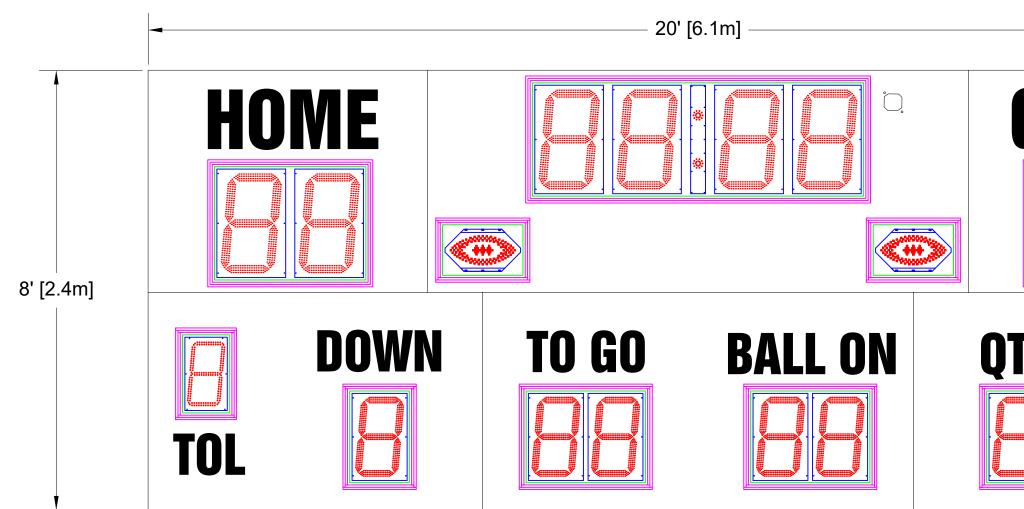
Overall size: 20' (W) x 8' (H) x 6" (D) Approximate Weight: 789 lbs Incoming Mains Power: (2x) 120VAC (+/-10%) 1 Phase, 2 Wire, 60Hz / 8 Amps. Requires an earth ground connection. Incoming Mains Power and Data Location: Behind the BALL ON Digit(s).
