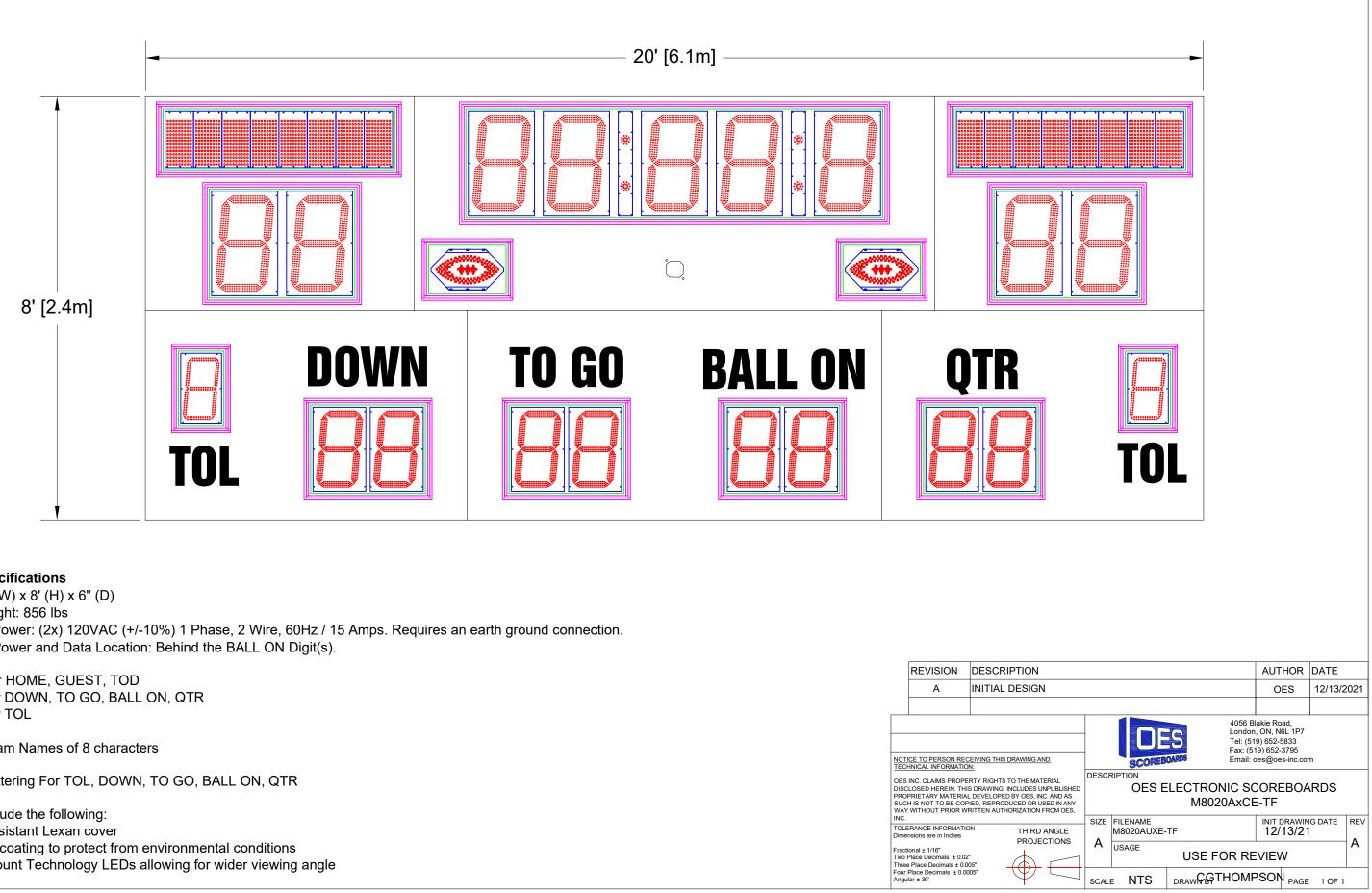
Overall size: 20' (W) x 8' (H) x 6" (D) Approximate Weight: 856 lbs Incoming Mains Power: (2x) 120VAC (+/-10%) 1 Phase, 2 Wire, 60Hz / 15 Amps. Requires an earth ground connection. Incoming Mains Power and Data Location: Behind the BALL ON Digit(s).
