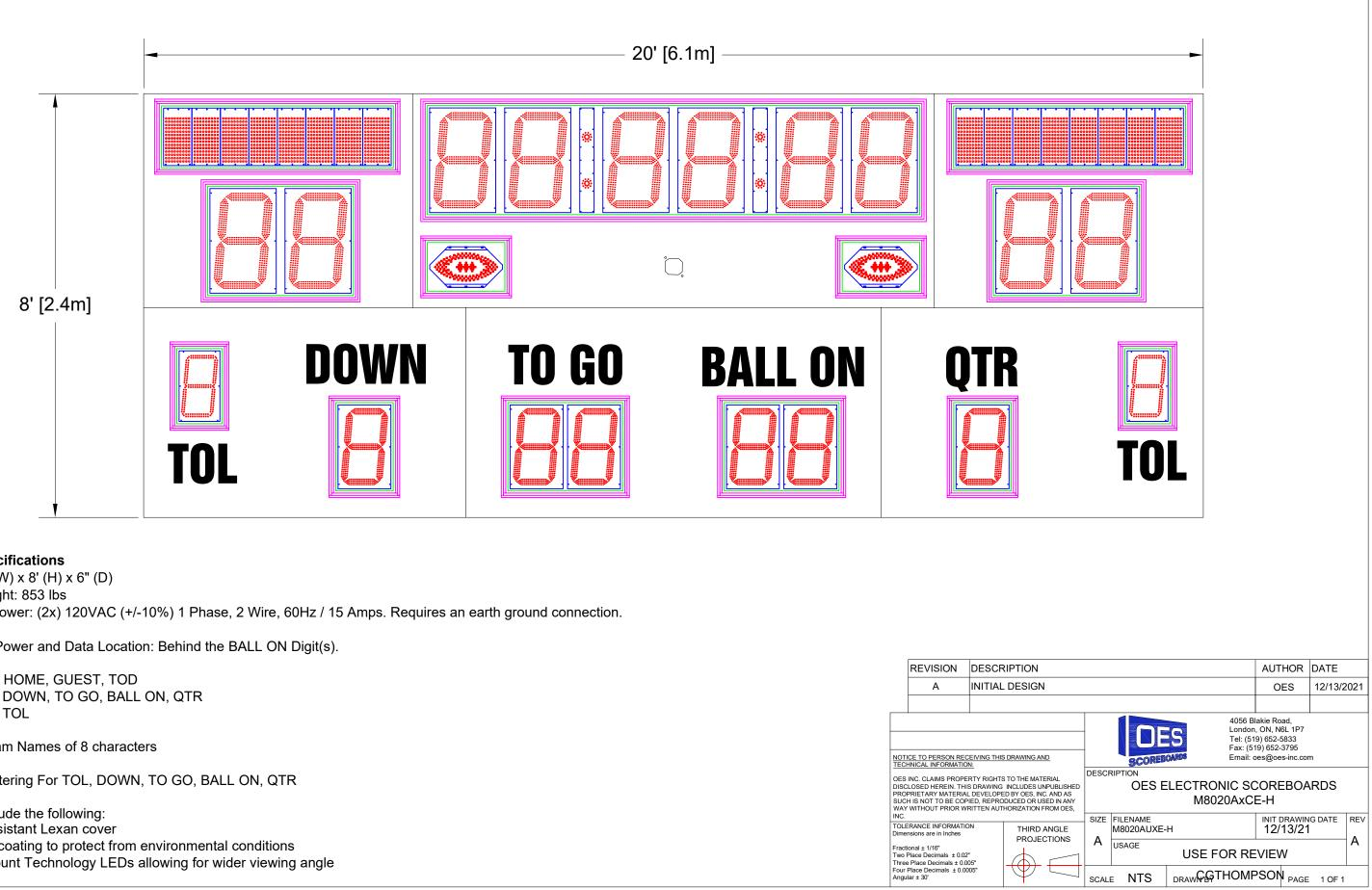
Overall size: 20' (W) x 8' (H) x 6" (D) Approximate Weight: 853 lbs Incoming Mains Power: (2x) 120VAC (+/-10%) 1 Phase, 2 Wire, 60Hz / 15 Amps. Requires an earth ground connection.
