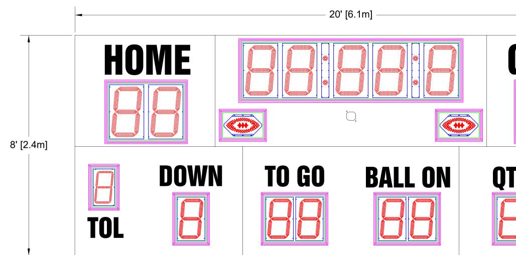
Overall size: 20' (W) x 8' (H) x 6" (D) Approximate Weight: 801 lbs Incoming Mains Power: (1x) 120VAC (+/-10%) 1 Phase, 2 Wire, 60Hz / 20 Amps. Requires an earth ground connection. Incoming Mains Power and Data Location: Behind the BALL ON Digit(s).
