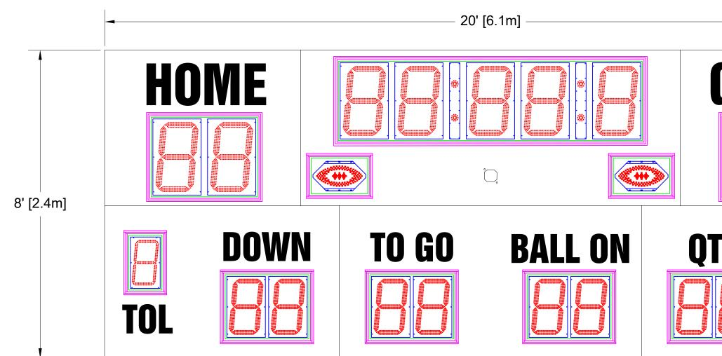
Overall size: 20' (W) x 8' (H) x 6" (D) Approximate Weight: 813 lbs Incoming Mains Power: (1x) 120VAC (+/-10%) 1 Phase, 2 Wire, 60Hz / 20 Amps. Requires an earth ground connection. Incoming Mains Power and Data Location: Behind the BALL ON Digit(s).
