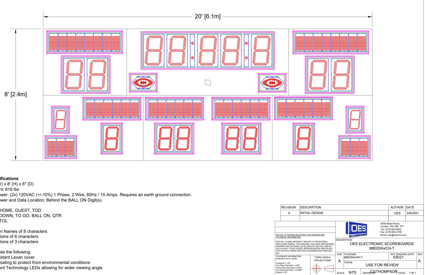
Overall size: 20' (W) x 8' (H) x 6" (D) Approximate Weight: 919 lbs Incoming Mains Power: (2x) 120VAC (+/-10%) 1 Phase, 2 Wire, 60Hz / 15 Amps. Requires an earth ground connection. Incoming Mains Power and Data Location: Behind the BALL ON Digit(s).
