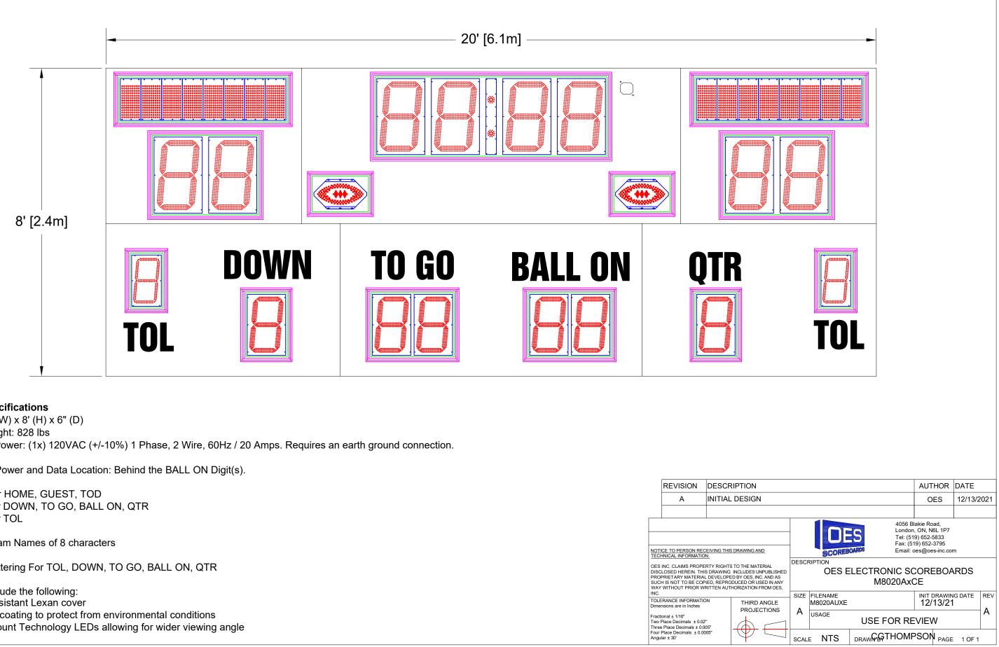
Overall size: 20' (W) x 8' (H) x 6" (D) Approximate Weight: 828 lbs Incoming Mains Power: (1x) 120VAC (+/-10%) 1 Phase, 2 Wire, 60Hz / 20 Amps. Requires an earth ground connection.
