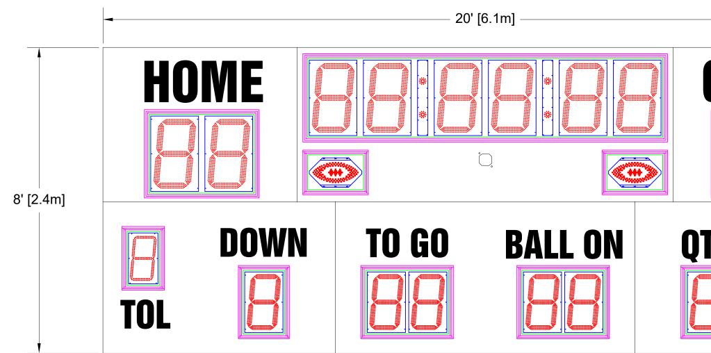
Overall size: 20' (W) x 8' (H) x 6" (D) Approximate Weight: 810 lbs Incoming Mains Power: (1x) 120VAC (+/-10%) 1 Phase, 2 Wire, 60Hz / 20 Amps. Requires an earth ground connection. Incoming Mains Power and Data Location: Behind the BALL ON Digit(s).
