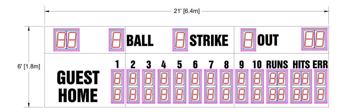
Overall size: 21' (W) x 6' (H) x 6" (D) Approximate Weight: 820 lbs Incoming Mains Power: (1x) 120VAC (+/-10%) 1 Phase, 2 Wire, 60Hz / 20 Amps. Requires an earth ground connection. Incoming Mains Power and Data Location: Behind the 8TH INNING Digit.
