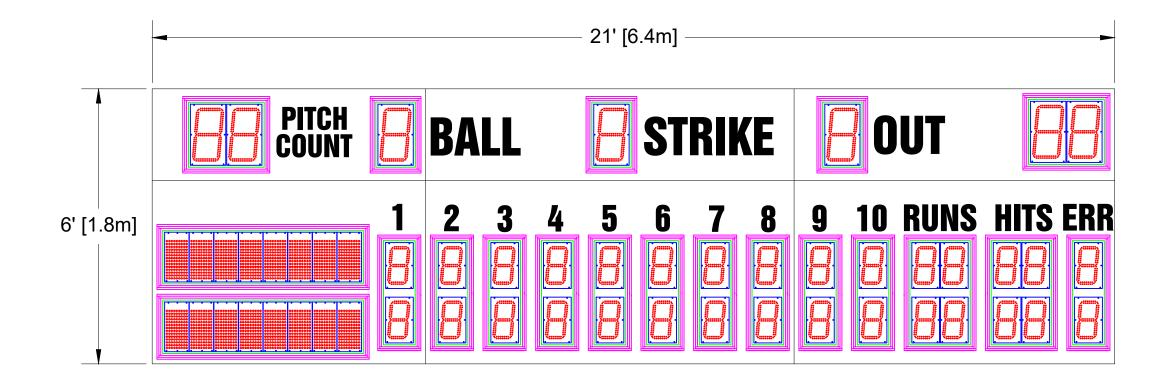
Overall size: 21' (W) x 6' (H) x 6" (D) Approximate Weight: 820 lbs Incoming Mains Power: (1x) 120VAC (+/-10%) 1 Phase, 2 Wire, 60Hz / 15 Amps. Requires an earth ground connection. Incoming Mains Power and Data Location: Behind the [8TH INNING] Digit(s).
