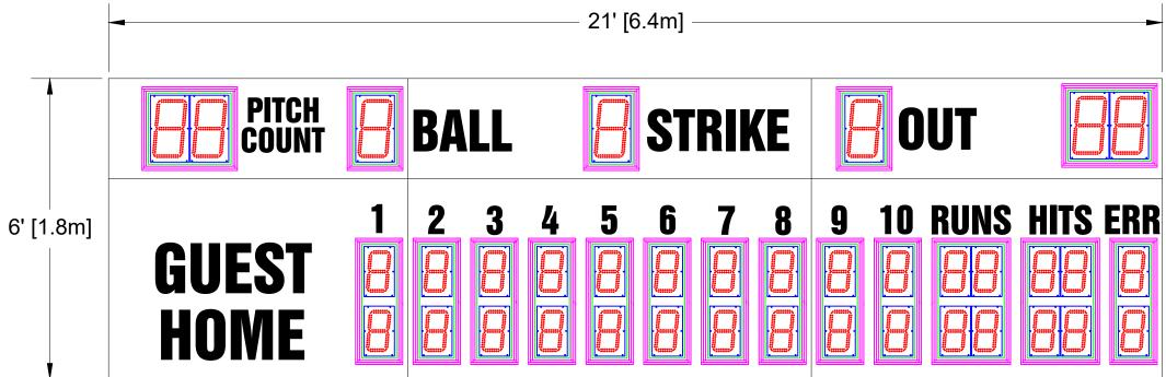
Overall size: 21' (W) x 6' (H) x 6" (D) Approximate Weight: 820 lbs Incoming Mains Power: (1x) 120VAC (+/-10%) 1 Phase, 2 Wire, 60Hz / 20 Amps. Requires an earth ground connection. Incoming Mains Power and Data Location: Behind the 8TH INNING Digit.
