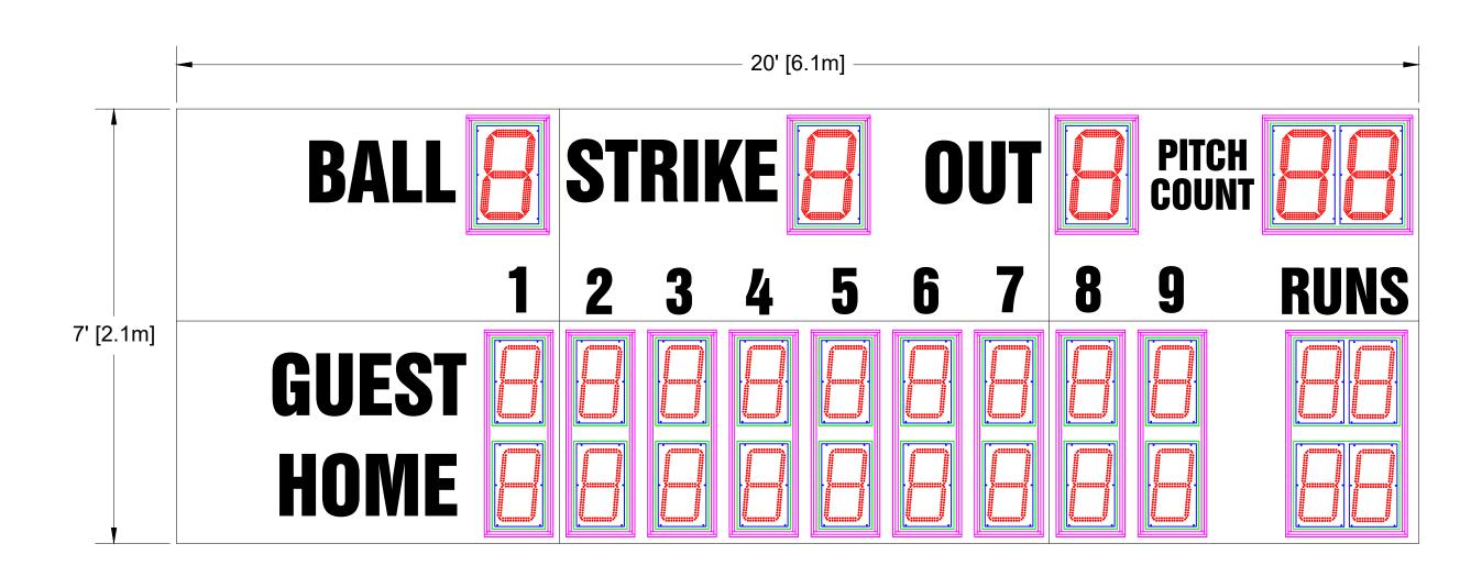
Overall size: 20' (W) x 7' (H) x 6" (D) Approximate Weight: 773 lbs Incoming Mains Power: (1x) 120VAC (+/-10%) 1 Phase, 2 Wire, 60Hz / 15 Amps. Requires an earth ground connection.
