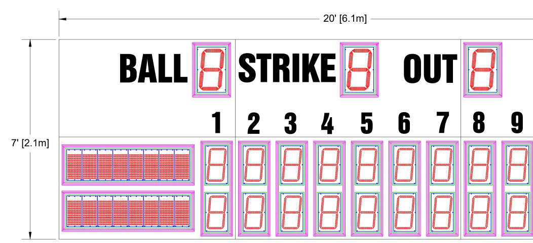
Overall size: 20' (W) x 7' (H) x 6" (D) Approximate Weight: 773 lbs Incoming Mains Power: (1x) 120VAC (+/-10%) 1 Phase, 2 Wire, 60Hz / 20 Amps. Requires an earth ground connection.
