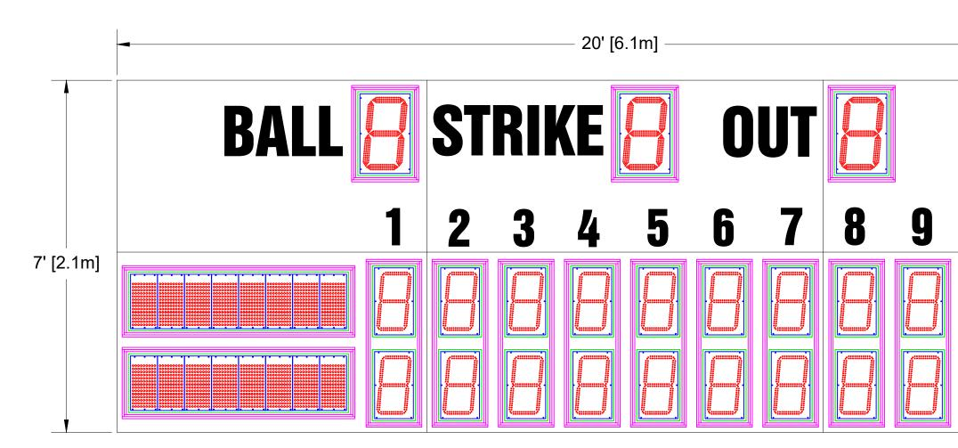
Overall size: 20' (W) x 7' (H) x 6" (D) Approximate Weight: 773 lbs Incoming Mains Power: (1x) 120VAC (+/-10%) 1 Phase, 2 Wire, 60Hz / 20 Amps. Requires an earth ground connection.
