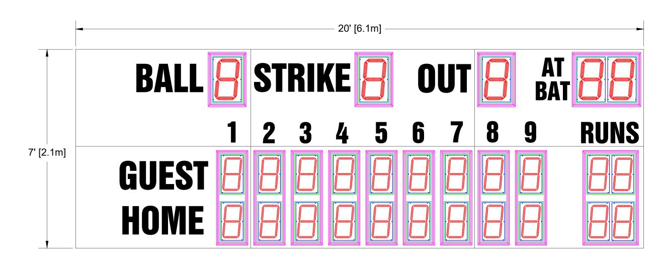
Overall size: 20' (W) x 7' (H) x 6" (D) Approximate Weight: 773 lbs Incoming Mains Power: (1x) 120VAC (+/-10%) 1 Phase, 2 Wire, 60Hz / 15 Amps. Requires an earth ground connection.
