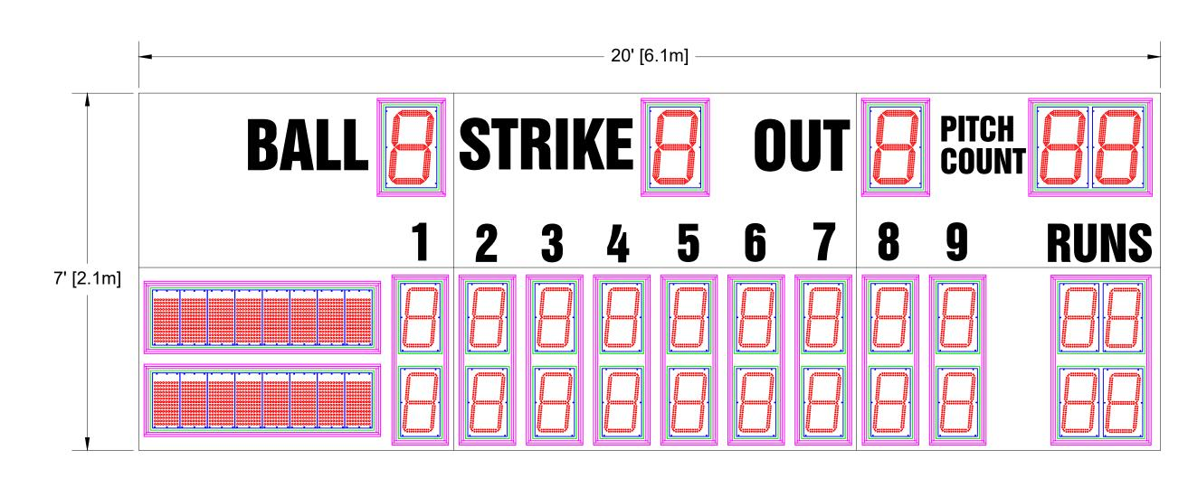
Overall size: 20' (W) x 7' (H) x 6" (D) Approximate Weight: 773 lbs Incoming Mains Power: (1x) 120VAC (+/-10%) 1 Phase, 2 Wire, 60Hz / 20 Amps. Requires an earth ground connection.
