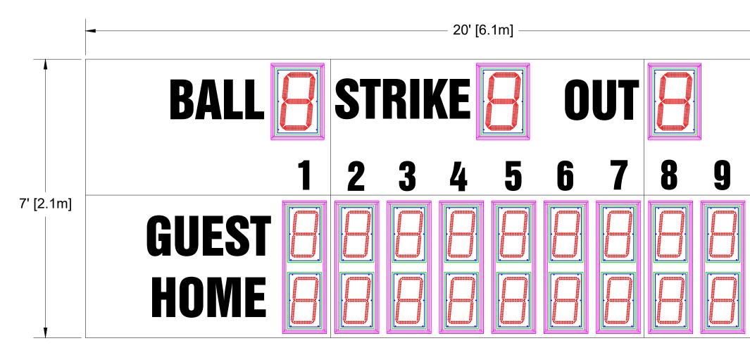
Overall size: 20' (W) x 7' (H) x 6" (D) Approximate Weight: 773 lbs Incoming Mains Power: (1x) 120VAC (+/-10%) 1 Phase, 2 Wire, 60Hz / 15 Amps. Requires an earth ground connection.
