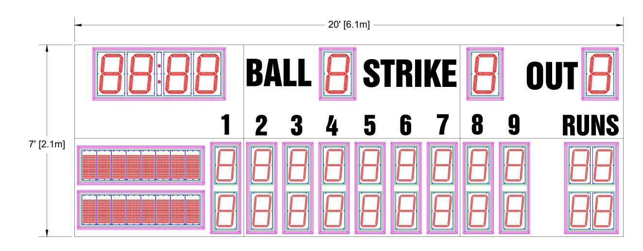
Overall size: 20' (W) x 7' (H) x 6" (D) Approximate Weight: 773 lbs Incoming Mains Power: (1x) 120VAC (+/-10%) 1 Phase, 2 Wire, 60Hz / 20 Amps. Requires an earth ground connection.
