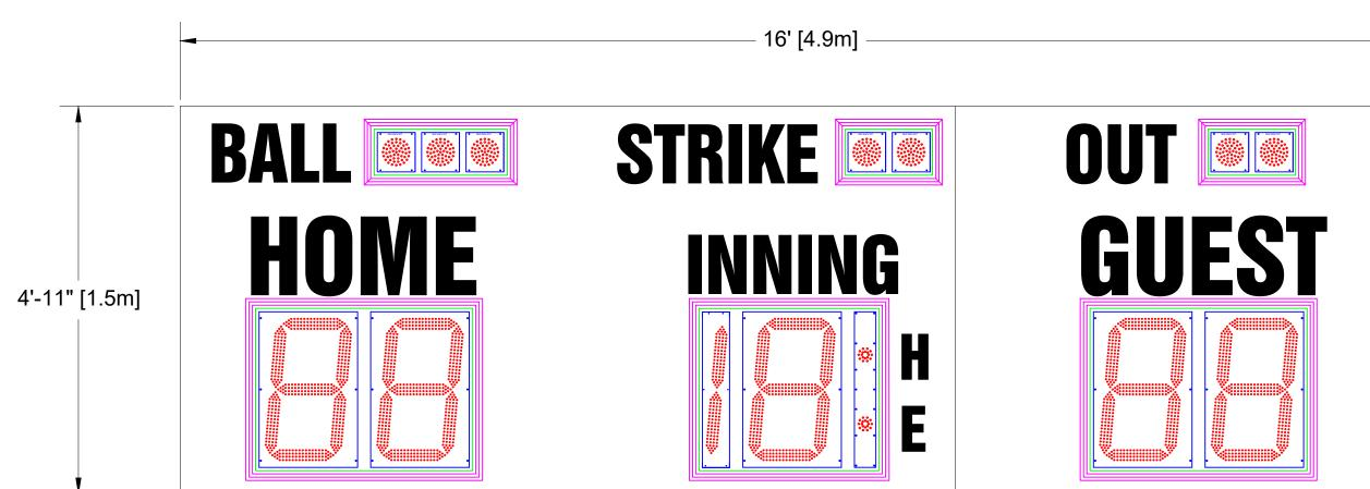
Scoreboard Specifications Overall size: 16' (W) x 4'-11" (H) x 6" (D) Approximate Weight: 467 lbs Incoming Mains Power: (1x) 120VAC (+/-10%) 1 Phase, 2 Wire, 60Hz / 10 Amps. Requires an earth ground connection. Incoming Mains Power and Data Location: Behind the INNING Digit.
