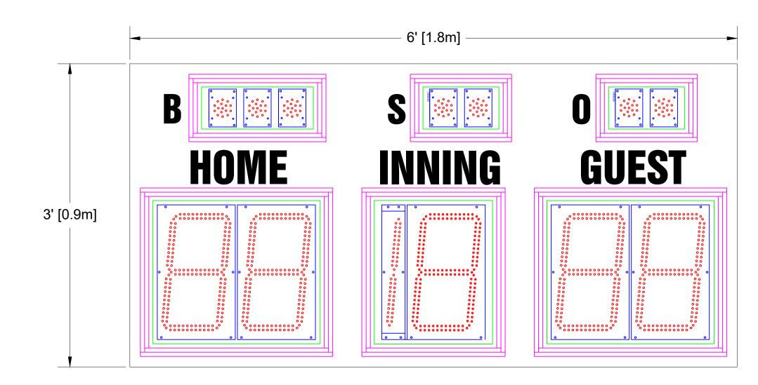
Scoreboard Specifications Overall size: 6' (W) x 3' (H) x 6" (D) Approximate Weight: 159 lbs Incoming Mains Power: (1x) 120VAC (+/-10%) 1 Phase, 2 Wire, 60Hz / 5 Amps. Requires an earth ground connection. Incoming Mains Power and Data Location: Behind the INNING Digit.
