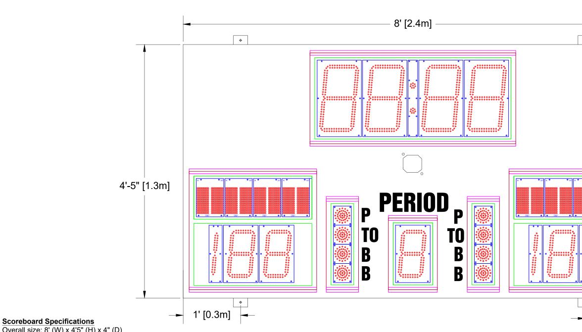
Overall size: 8' (W) x 4'5" (H) x 4" (D) Approximate Weight: 167 lbs Incoming Mains Power: (1) 120VAC (+/-10%) 1 Phase, 2 Wire, 60Hz / 8 Amps. Requires an earth ground connection. Incoming Mains Power and Data Location: TOP of the Scoreboard.
